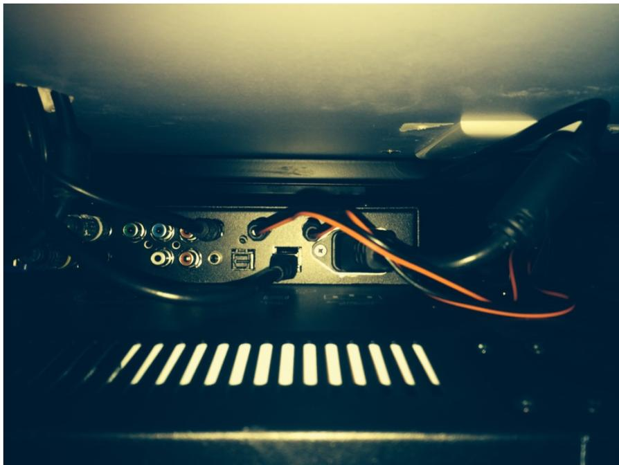
**Under view of the Touchscreen showing the speaker cables (red and black) connected.**
